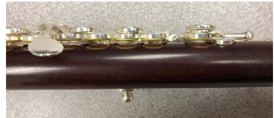
Fig. 4: Venthole remains closed when C# tonehole is open
